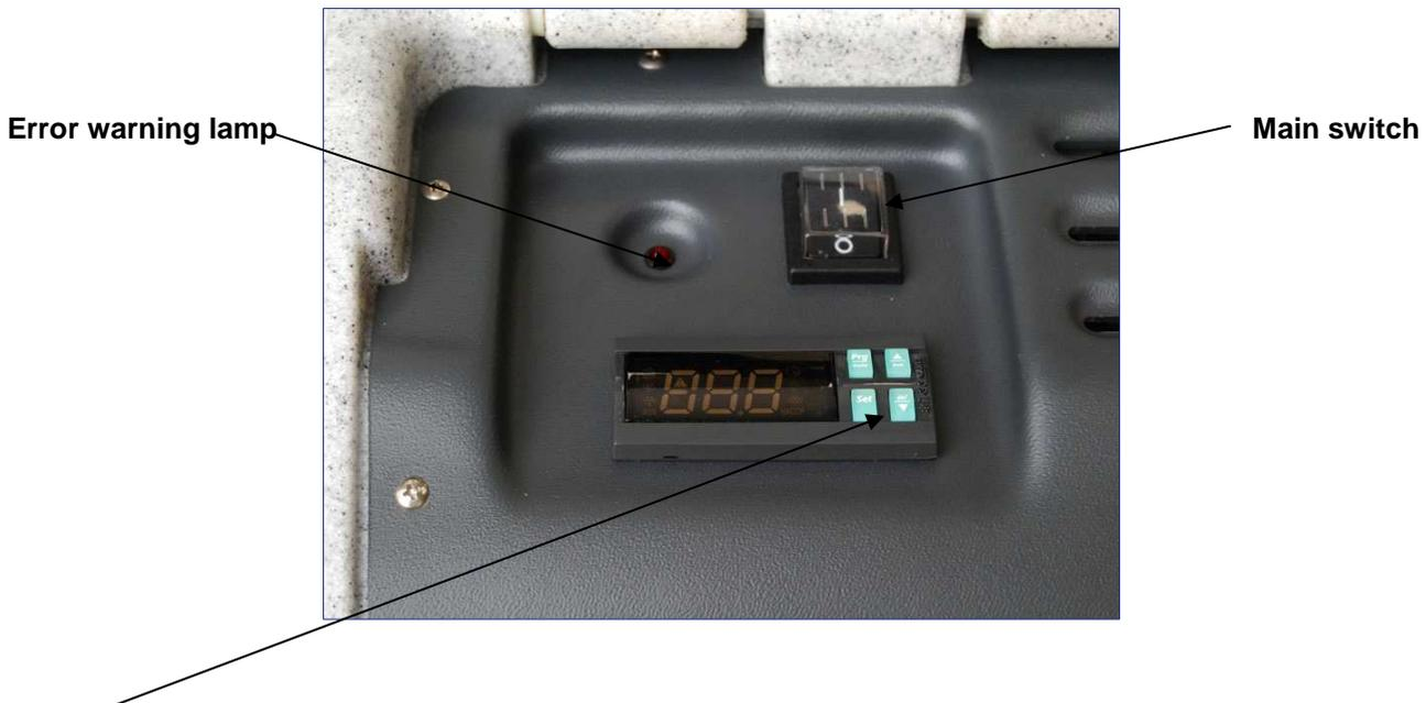
**Digital electronic thermostat** with incorporated alarm: microprocessor operating, with 4 switches, allowing the control of all the refrigerator functions (maintaining of the adjusted temperature, compressor and fans functioning). The internal temperature is displayed with a LED display, with red colour, bright indication and an accuracy of 1°C.
