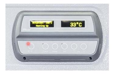
**Microprocessor controller** with OLED display. Temperature and time are entered via touch button below the display. Time values can be set in minutes from 1 to 999.
