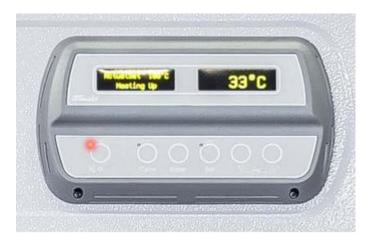
**Microprocessor controller** with OLED display. Temperature and time are entered via touch button below the display. Time values can be set in minutes from 1 to 999. The set time corresponds to the actual operating time. Therefore, the heating time does not need to be estimated and added.
